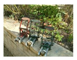
A single stage Kismet Baby is shown next – restored to concourse/display condition. This is a backward pumping design with the non-return valve behind a brass bolt at the rear air outlet point.
