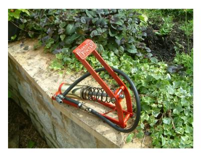
An interesting variation on the normal single stage design is where two compression chambers are used in parallel – basically to double the volume of air compressed on each stroke. Each chamber compresses the same volume of air to the same pressure.
