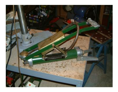
The mechanism by which the two pistons are simultaneously activated by one down stroke of the pedal can be seen. Also, the return spring (a parallel coiled tension spring) is shown. Coiled tension springs in vintage pumps are quite rare – the only other common examples being in the Dunlop Major and Standard.
