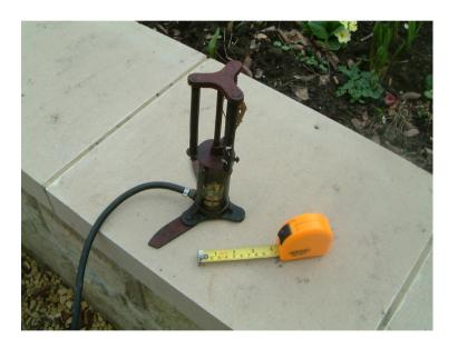
The working principle is very simple – pressing the foot down on the platform at the top drives a piston down the barrel underneath. There is a NRV in the hose-tail at the outlet at the bottom. There are three coiled compression return springs on the vertical supports. The swept volume in the barrel at each stroke is quite small – so lots of strokes needed to get up pressure.
